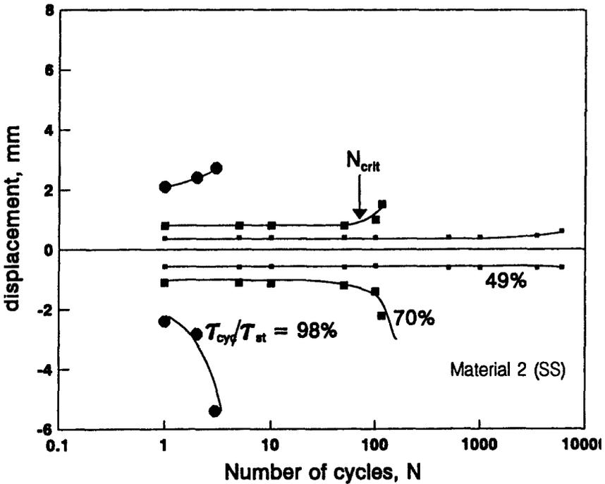
Fig. 7. Evolution of shear displacements in terms of the number of applied load cycles for different stress amplitudes
