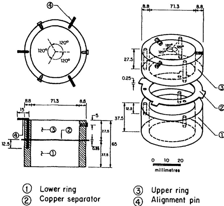
Fig. 1b. Direct Shear rings
