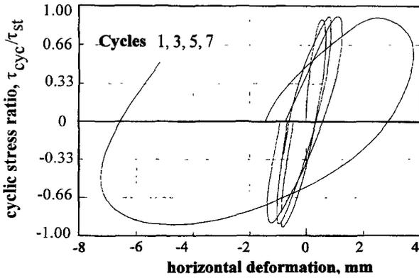
Fig. 5. Typical cyclic stress–deformation curve (material 1, soil-on-soil test)
