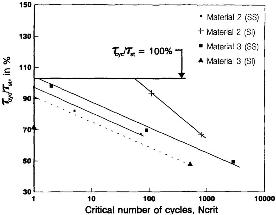
Fig. 8. Relationship between the critical number of cycles and the normalized stress amplitude
