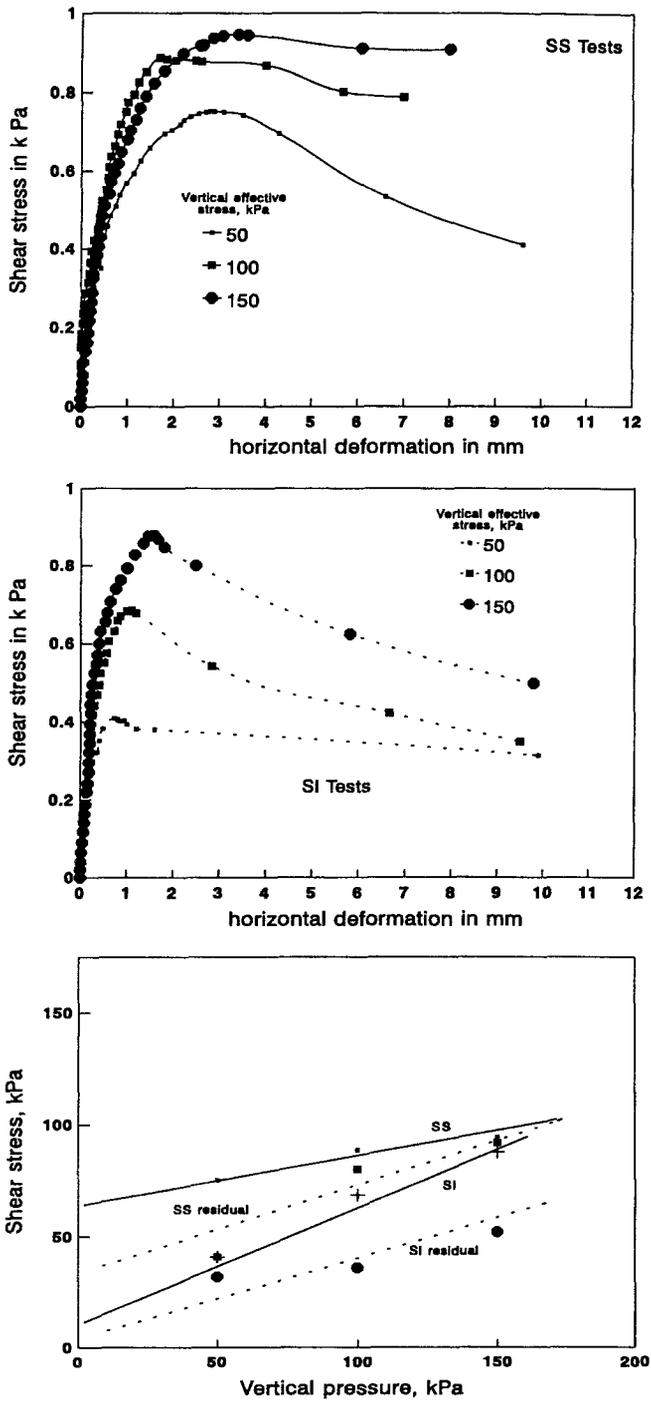
Fig. 3. Peak and residual strength envelopes from static direct shear tests
