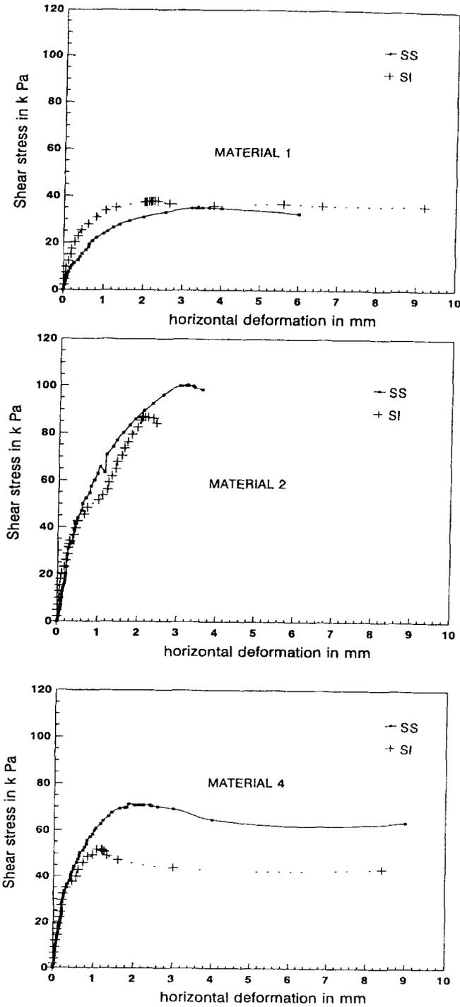
Fig. 2. Stress–deformation curves from static soil-on-soil (ss) and soil-on-interface (SI) tests
