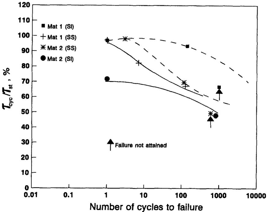
Fig. 6. Relationship between the number of cycles to failure and the cyclic stress amplitude
