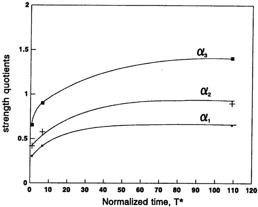
Fig. 10. Evolution of the strength quotients with normalized time
