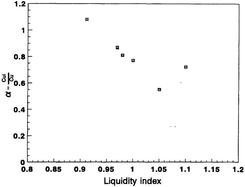
Fig. 4. Experimental relationship between the adhesion coefficient and liquidity index
