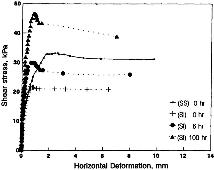
Fig. 9. Results of static direct shear tests on remoulded clays with different consolidation times
